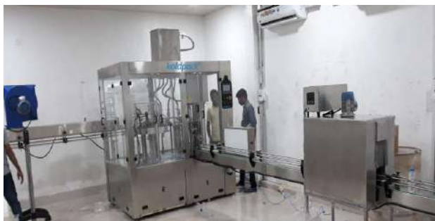
Pilot scale water bottling unit of 1000 bottles per hr capacity
