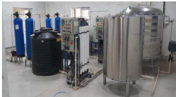
Indigenous pilot scale membrane system of 1200 L/h capacity
