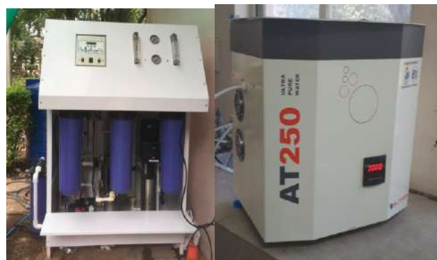
DM water system of 200-500 L/h (left) and 40-60 L/h capacity (right)
