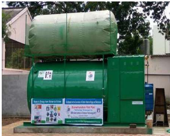
Biogas plant (250 kg/day) installed at CSIR-IICT, Hyderabad
