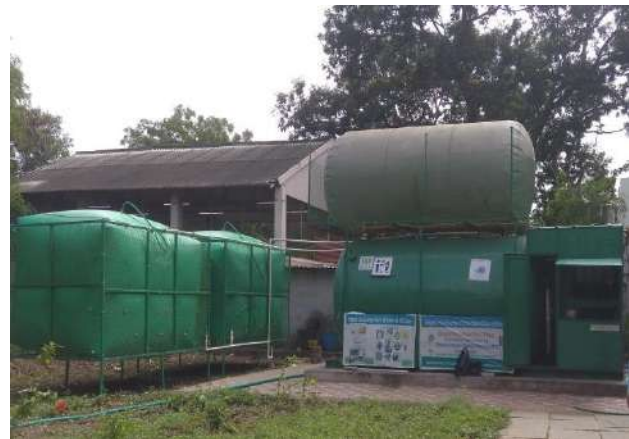
Biogas plant (250 kg/day) installed at CSIR-IICT, Hyderabad
