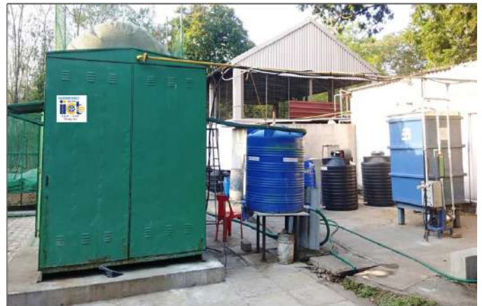
Aerobic Moving Bed Bioreactor (AMBBR) + side stream NF
