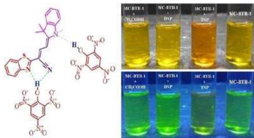
Fig. 21 MC-BTH-1 conjugate displaying sensing property towards picric acid
