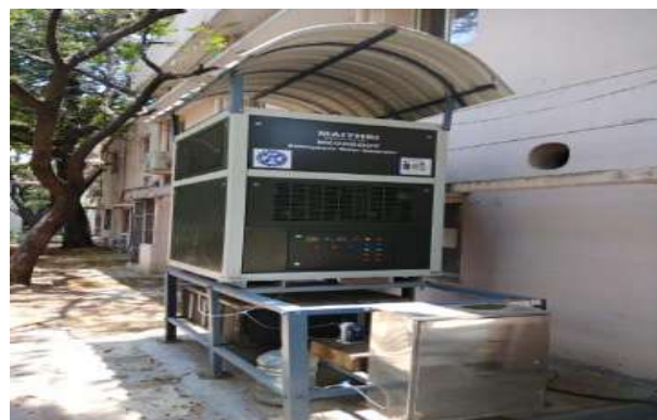
Atmospheric Water Generator Demonstration Unit of 1000 Lit/day capacity installed by CSIR-IICT & Maitri Aquatech Pvt. Ltd. at IICT campus
