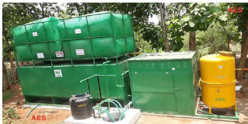
Full scale biogas plant for the treatment of food waste based on AGR at Rourkela, Odisha
