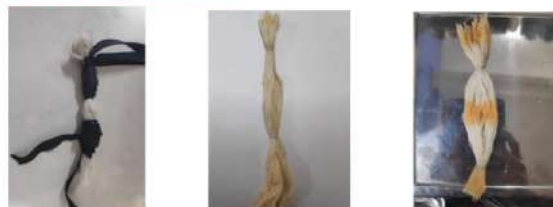
Before Dyeing After 10 min of heating at 70°C After 10 min of Cavi-Dyeing at 25 °C
